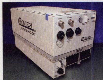
3. Model XTD-750KHE is an antenna-mount TWT with 750 W peak output power from 13.75 to 14.50 GHz. [Photo courtesy of Comtech Xicom Technology ( www.xicomtech.com )]
