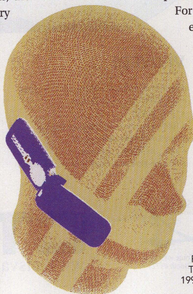
9. The embedded antenna in a mobile phone can be evaluated by means of an FDTD-based EM simulation.
