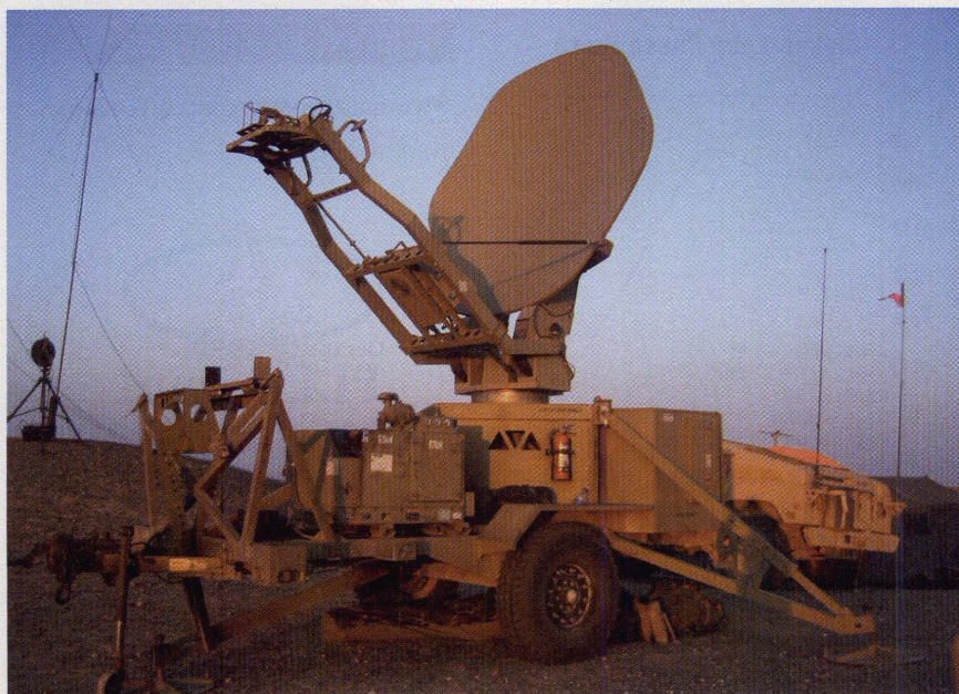
1. This satcom trailer, powered by a Ku-band TWTA from MCL, was used for mobile satcom applications in Iraq during Operation Iraqi Freedom. [Photo courtesy of MCL, Inc. ( www.mcl.com ).]
