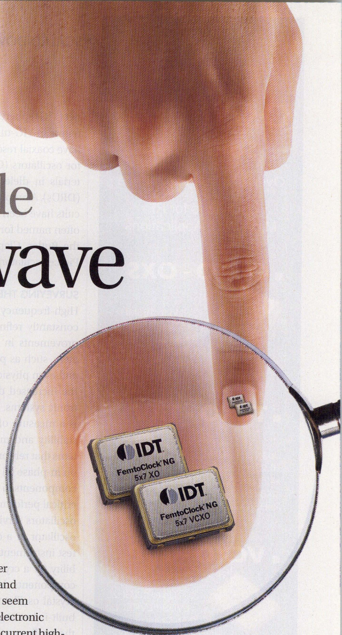
1. These crystal oscillators and VCXOs operate through 1300 MHz in packages measuring only 5 x 7 mm. [Photo courtesy of Integrated Device Technology ( www.idt.com ).]
